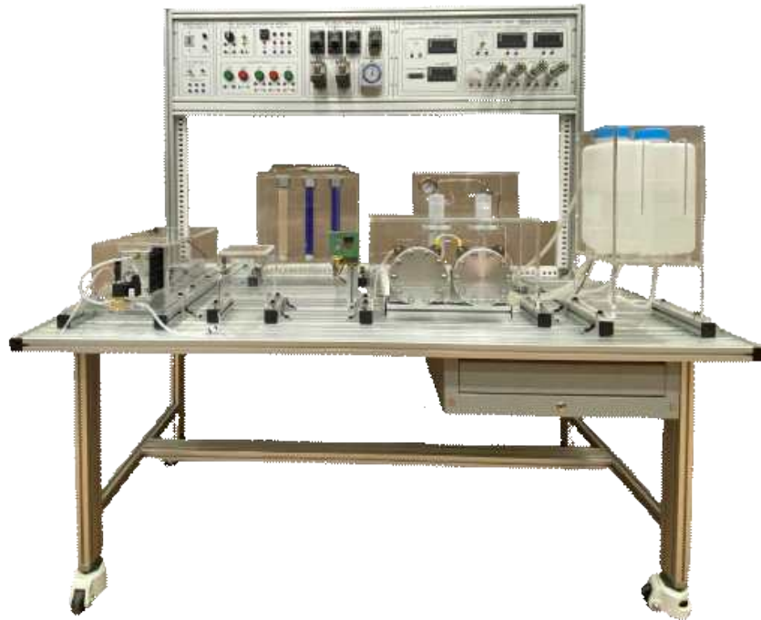
Experimental equipment for hydrogen fuel cell power generation using electrolysis (KTE-7000HS)
